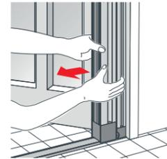
**6.1** Hold the folded mesh profile of the mosquito screen with your hands and pull towards the side guide to separate it from the structure. It's easier to separate it from the bottom. Position the mosquito screen along the side guide.
