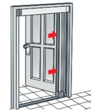
**5.5** Push the screen with the anchor plate to the installation position (folded mesh profile) strongly so that the anchor plate adheres well to the bottom of the screen touching the bottom guide.
