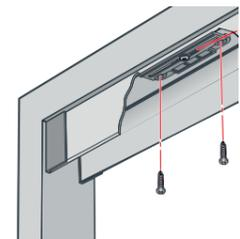
**9.3** Install the second pleated mosquito screen unit above the thread regulator.
