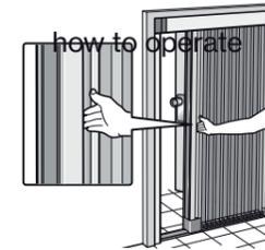
**Note:** do not add any parts such as the handle, etc., to the product with screws, as this may damage the opening and closing operation.
