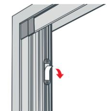
**5.2** Insert the mosquito screen and the side guide (joined together with the magnet) into the top guide. The side guide should be inserted into the opening in the largest end of the top guide and the bottom of the screen should be placed over the lower fixed guide.
