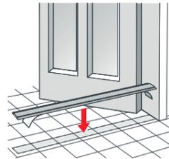
**4.2** Remove the white tape from the double-sided tape and press it to the ground strongly in line with the marked line. Be sure to press it toward the side of the folded mesh profile and make sure that there is more than 7.5 mm of space on each side of the side guide.
