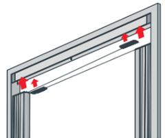
**9.4** Install the second pleated mosquito screen unit above the thread regulator.
