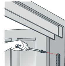
**6.2** Screw the anchor plates firmly with the screws as they are only temporarily stuck with the double-sided tape.
