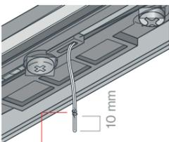
**Note:** make sure that the thread regulator is not installed in the upper rail screw. If this is the case and you cannot avoid it, cut the thread and make a double knot leaving about 10 mm at the end of the thread as shown in this image.
