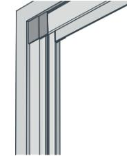
**5.6** Secure the side guide with the anchor plates.
