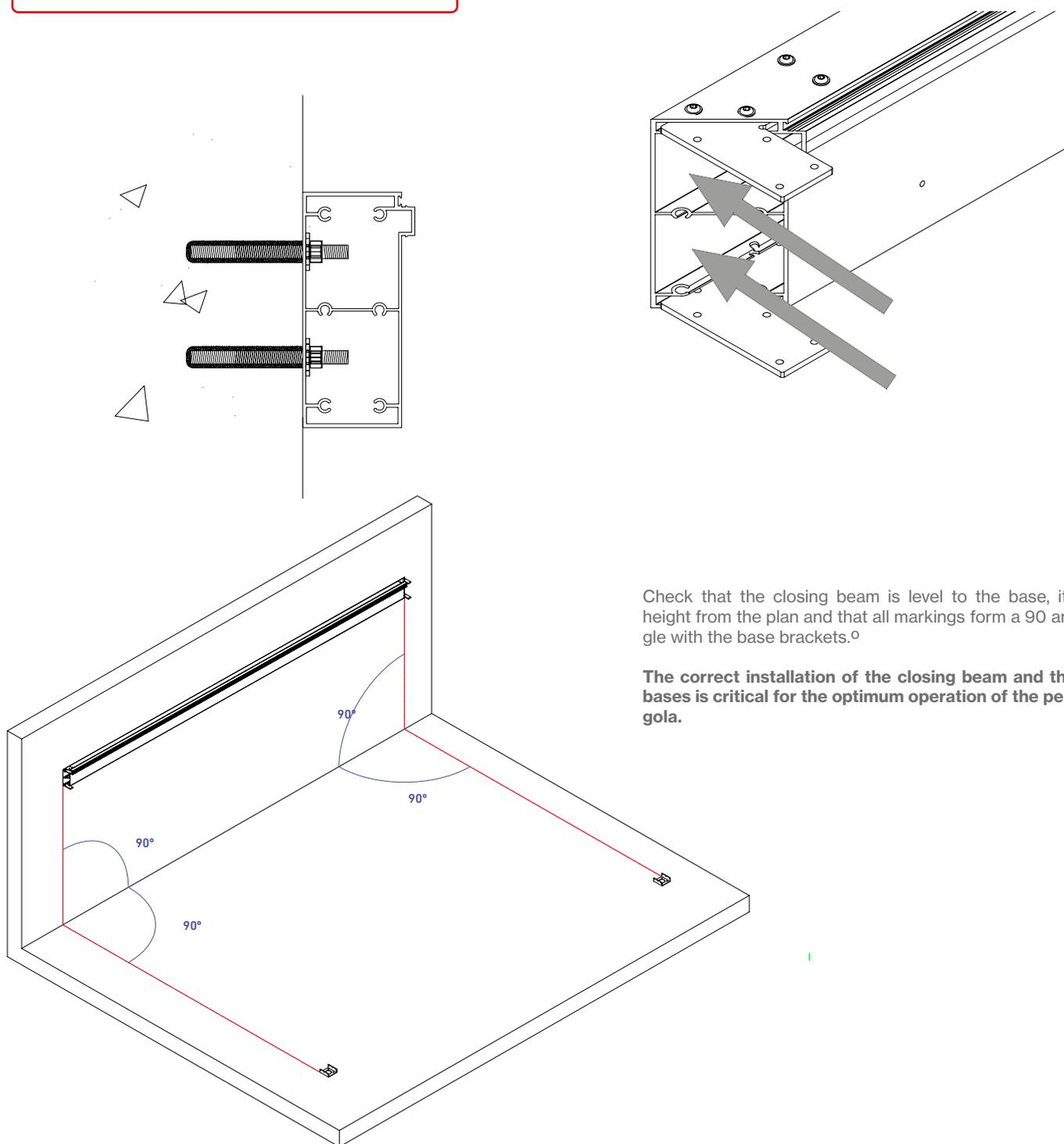
Check that the closing beam is level to the base, its height from the plan and that all markings form a 90° angle with the base brackets.°
