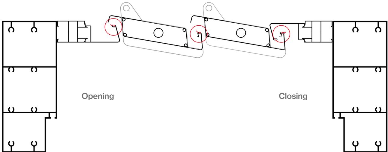
Installing rubber on the clippable opening gutter.
