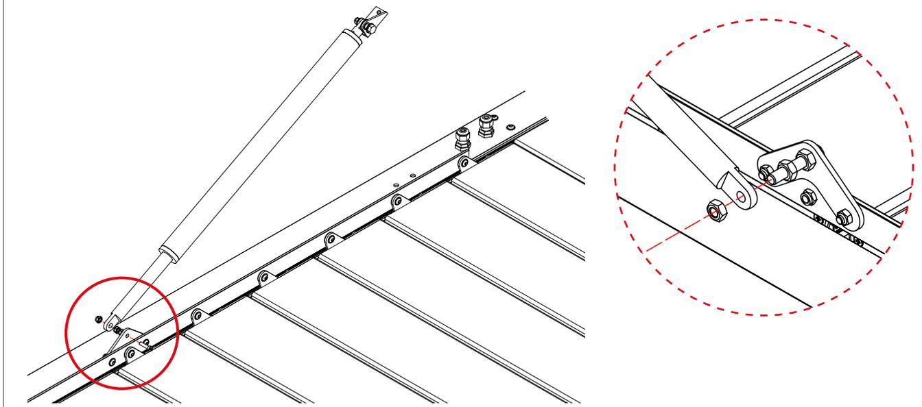
3. Move the motor opening the pergola until the bracket can be screwed on the beam threaded holes.
