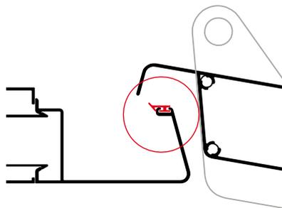
Installing rubber on the last slat.
