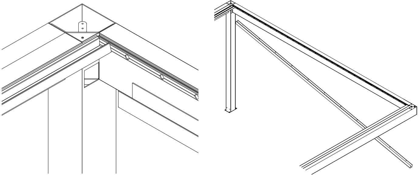
Check that all the "U" profile holes match the M6 machined ones on the beam. If all of them match, apply the sealant between the "U" profile and the beam after screwing the profiles with the USL (ISO 7380) A2x16 screws.
