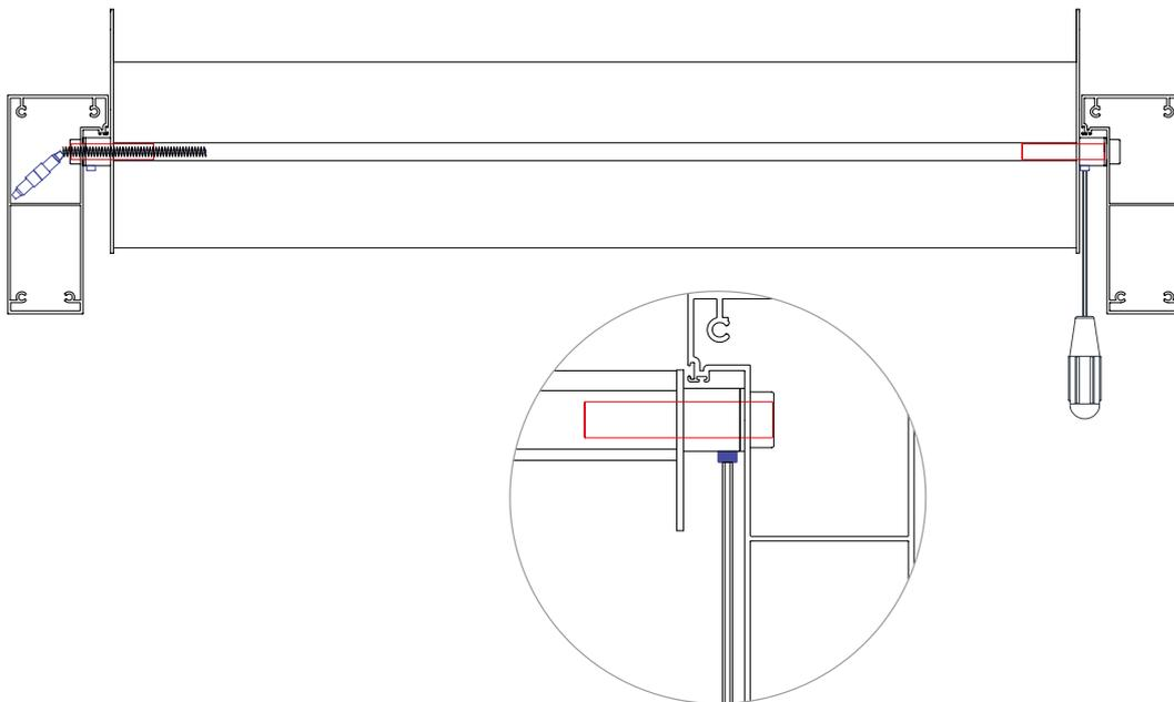
Using a N° 4 Allen key, pull back the axle until it stops in the grooved hole.
