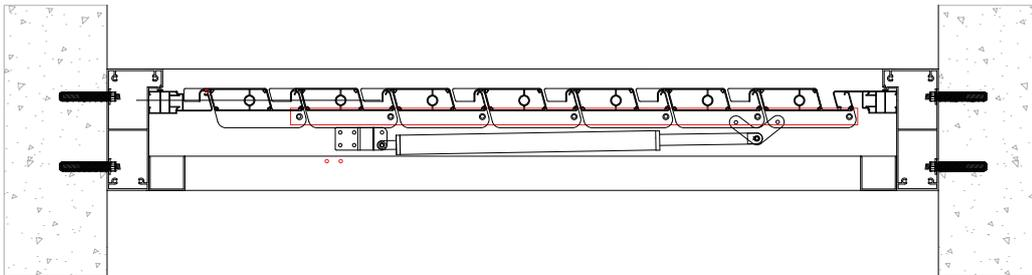
3. Mount the nut on the transmission plate stud so the motor does not come out (B).
