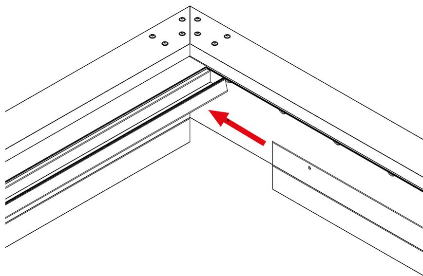
Check that all the "U" profile holes match the M6 machined ones on the beam. If all match, apply sealant between the U-profile and the beam and around the screw holes, then screw the profiles together using ULS (ISO 7380) A2 M6x16 screws.
