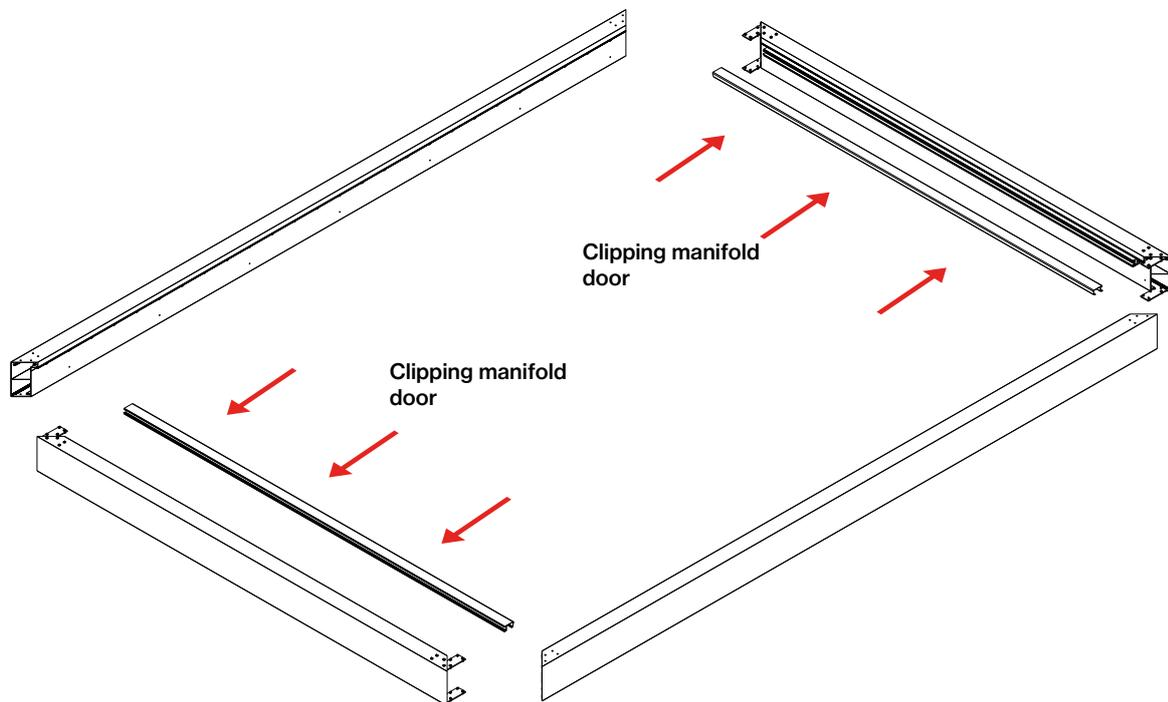
Apply sealant supplied between the mating faces of the clip-on siding on the **opening** and **closing** beam and respective manifolds.
