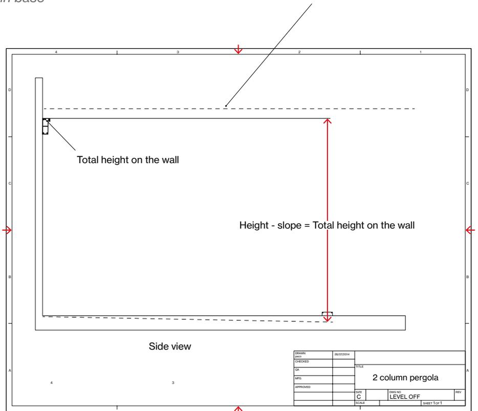
Position the column bases according to the measurements on the plan and the foundation slope, considering that the columns must form a 90° angle with the wall where the pergola is going to be installed.
