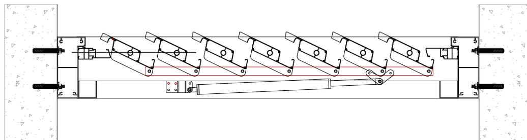
4. Finally we reinstall the motor support in the “U” profile with its 2 screws (A).
