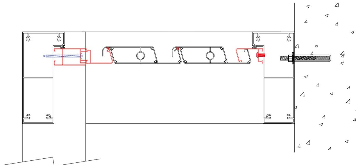
Check that all the "U" profile holes match the M6 machined ones on the beam. If all of them match, apply the sealant between the "U" profile and the beam after screwing the profiles with the ULS (ISO 7380) A2 M6x16.
